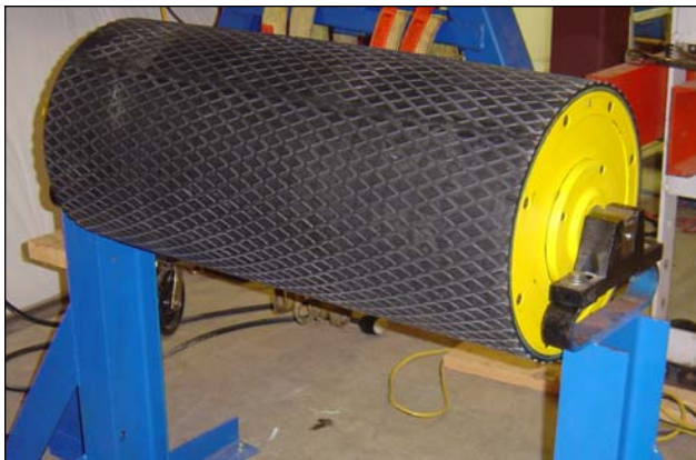
10 HP Motorized Pulley is fully tested before shipment.
