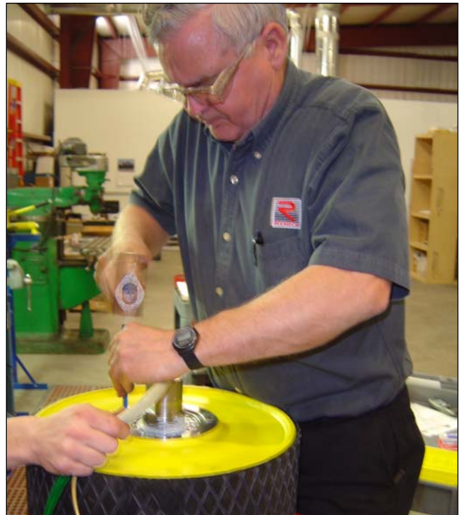
Merle Graham puts finishing touches on Rulmecca Corporation's first 400M Motorized Pulley, designed for 460v/3ph/60Hz power supply to drive a steel mill's 36" wide conveyor belt at 240 fpm.
