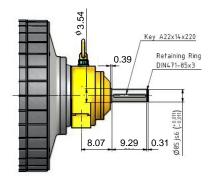
\* All dimensions are in imperial units, except for brake shaft diameter, key, and retaining ring, which are metric.
