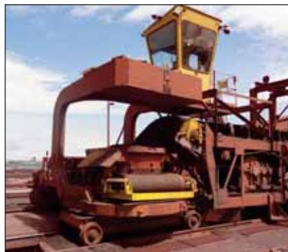
Pulleys at the head and tail positions, with electronic load-sharing, eliminated the problem on this reversing shuttle belt, which feeds the 60 ship loader surge bins. A close up of the west end drive is shown.
