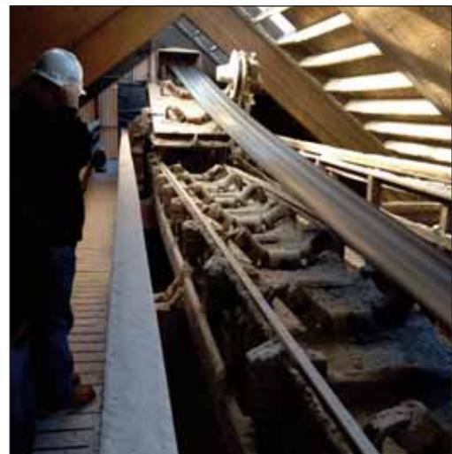
stainless steel 20 HP model 400M Motorized Pulleys in the head and tail positions.
