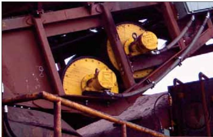
After upgrading three bucket wheel iron ore reclaimers with a 200 HP dual drive system on the discharge conveyor, this Great Lakes rail-to-ship transfer terminal extended discharge belt life by decreasing slack side tension. A serpentine belt wrap angle of 420° produced by the two 31.5" diameter Motorized Pulleys made this possible. More than ten years of successful operation have confirmed that belt life has been extended.
