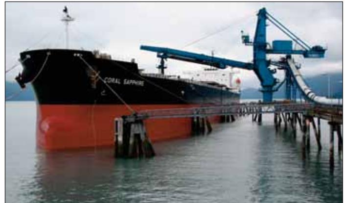
This Alaskan rail-to-ship transfer terminal installed a 75 HP 24.8" diameter Motorized Pulley in the ship loader shuttling boom conveyor when they upgraded the machine to handle 2,000 tph of coal. Faced with frigid conditions, the operator chose the optional anti-condensation heater, which maintains a constant warm temperature within the pulley shell when the machine is idle. Other operators use "trickle voltage" heating to serve the same purpose.
