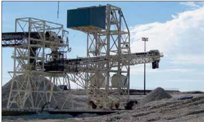
Belt wrap was increased from 180° to 360° at this western US trona mine by the adding a 50 HP 24.8" diameter Motorized Pulley to the head of this 30 year old radial stacker. It eliminated slippage of the 100 HP tail drive during rainy conditions. The 2,400 lb. Motorized Pulley replaced a 3,200 lb. idler pulley.
