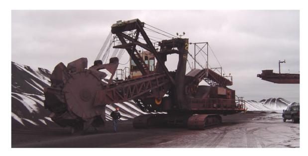
Photo shows one of three 40 year old bucket wheel reclaimers outfitted with 100 HP Rulmeca Motorized Pulleys. In addition to improving reliability, dual drive system on tail conveyor extended belt life since its 2004 installation.
