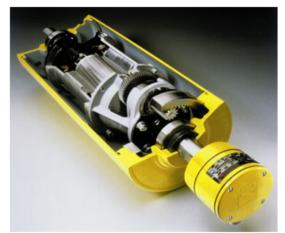
Cut-away photo shows Rulmeca's AC motor and gearbox hermetically sealed within the oil-filled Motorized Pulley shell, offering high reliability and low maintenance requirements.
