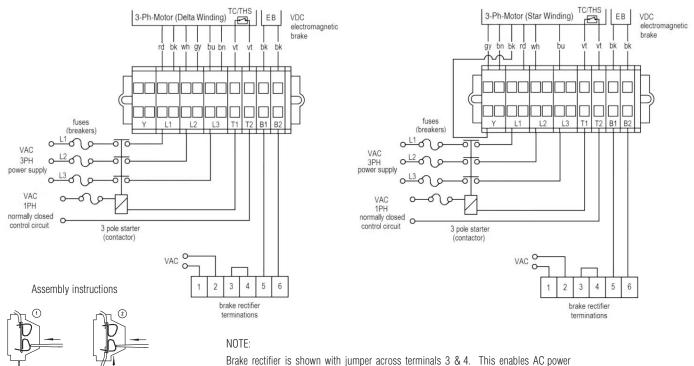
connecting an external switch to terminals 3 & 4.
