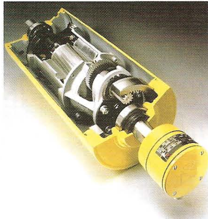
Rulmeca's motorized pulleys can make booster or temporary drives for longwall conveyors because the motor and gearbox are hermetically sealed within the pulley shell.
