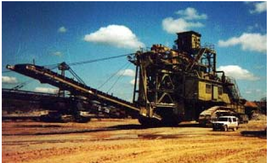
Fig. 2: One of three mobile primary crushers installed in an open pit continuous limestone mine in Rubeland, Germany in 1983. This mobile crusher still uses a 50 HP tail-mounted motorized pulley to drive elevating transfer belt.
