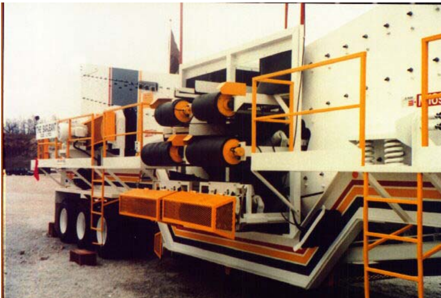
Fig. 6: Two 3 HP drives for 24 inch "cross belts" and four 4 HP drives for 30 inch "cross belts" were installed in this mobile screen central transfer point. Enclosing motors and gearboxes within motorized pulley shells enabled this Canadian manufacturer to simplify the design, assembly, and maintenance of this rig.
