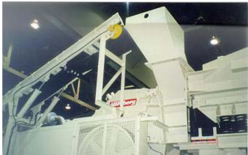
Fig. 12: This mobile crushing/screening plant manufacturer has used Interroll motorized pulleys as standard equipment in the United States and Canada for ten years.
