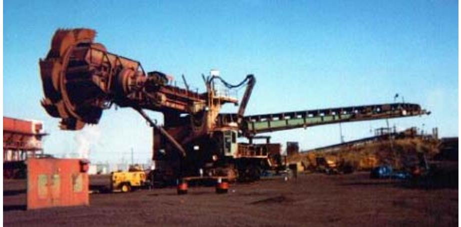
Fig. 1: German-engineered bucket wheel stacker reclaimer installed at a rail-to-ship transfer terminal for taconite pellets in Escanaba, Michigan in 1980. This machine still uses 200 HP motorized pulleys to drive boom and tail belts.
