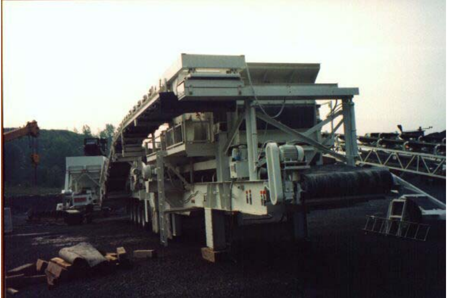
Fig. 8: Close-up of 800 tph pivoting screen feed belt (pinned in transport position.) US highway clearance requirements limited head pulley maximum width to 50 inches. 25 HP drive pulley width would have been 60 inches. Therefore, two 15 HP drives were used (at head and tail.)
