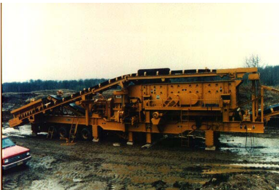
Fig. 7: Overview of 800 tph mobile crushing/screening plant designed by US subsidiary of Swedish equipment manufacturer. US highway restrictions limited this rig to 13'-6" high by 12'-0" wide. Driving the 36" wide elevating screen feed belt at 384 fpm required 23.5 HP. Equipment designer selected Interroll's "dual drive" arrangement.
