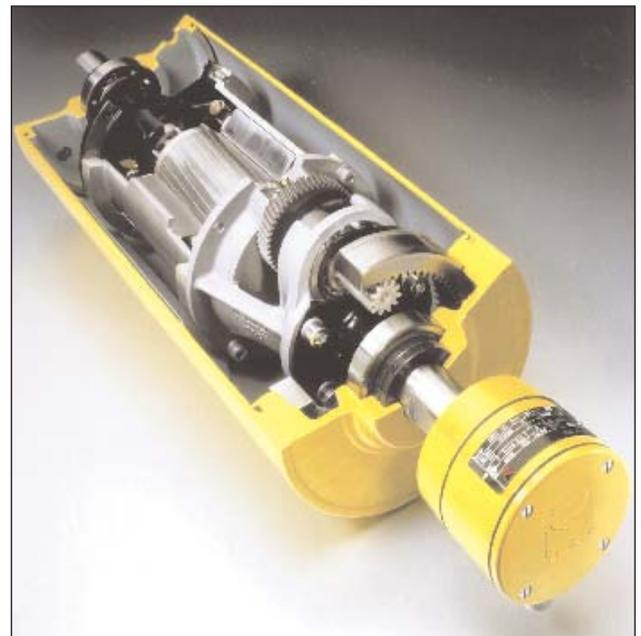
*Rulmecca Motorized Pulleys save valuable space because the drive's motor and gearbox are enclosed within the pulley shell. Operator safety is improved by the unit's "dead shaft" and enclosed drive design that eliminates pinch points.*
