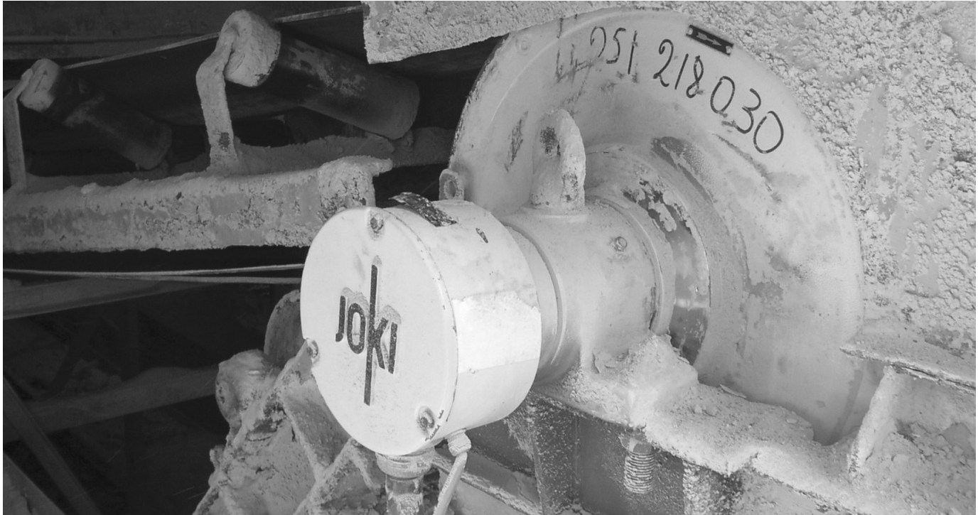
Aggressive & abrasive potash application located in the desert. Features: Re-greasable IP66/67 seals, insulation class H motor, NO maintenance and operating through Frequency Converter.
