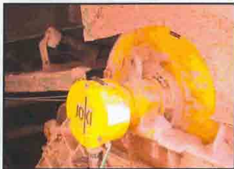
Ten-year-old JOKI Motorized Pulley drives 750 tph inclined conveyor belt at phosphate plant.
