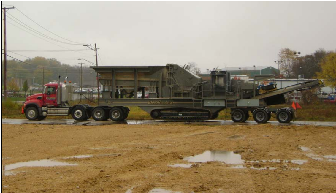
5066 Tracker features quick and easy transport capability using built-in 3 axle bogey and requires no escort.
