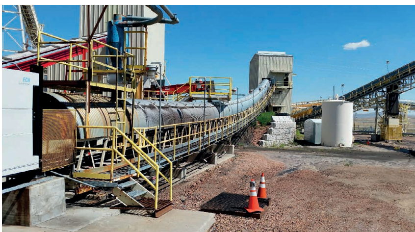
Figure 3. Silo reclaim conveyor #130 transfers coal from three silos to an overland conveyor or a truck loader on a 54 in wide belt at 600 ft/min.
