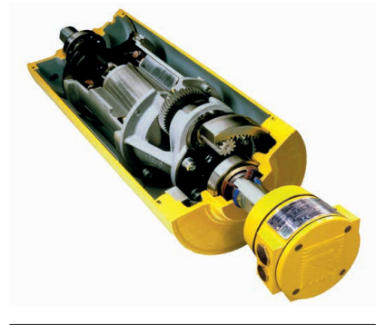
Figure 5. Motorised pulley hermetically seals motor and gearbox within oil-filled pulley shell.
