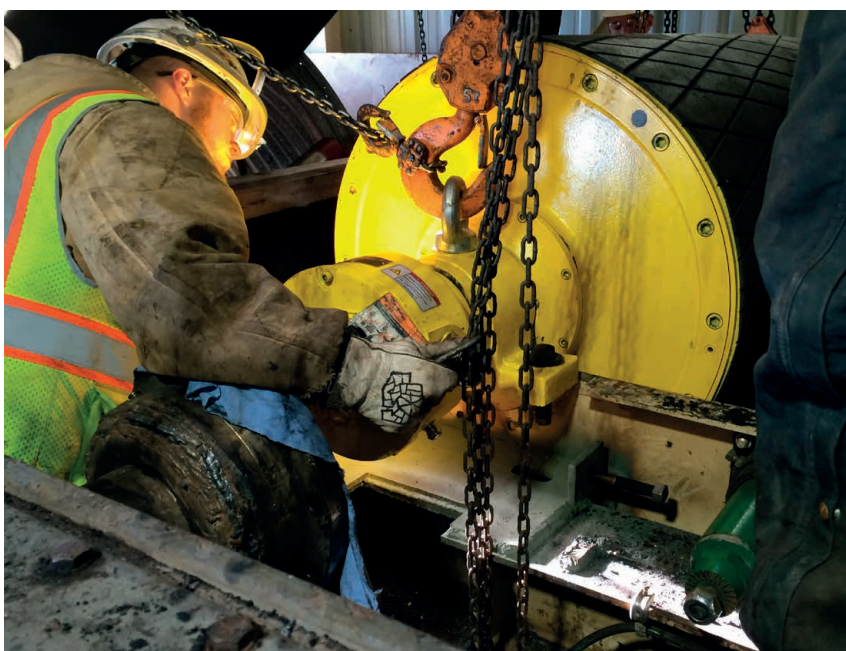
Figure 4. Model 800HD Rulmeca motorised pulley at 180 hp with face width of 61.02 in., belt speed of 600 ft/min. and full ceramic lagging was installed in one shift.
