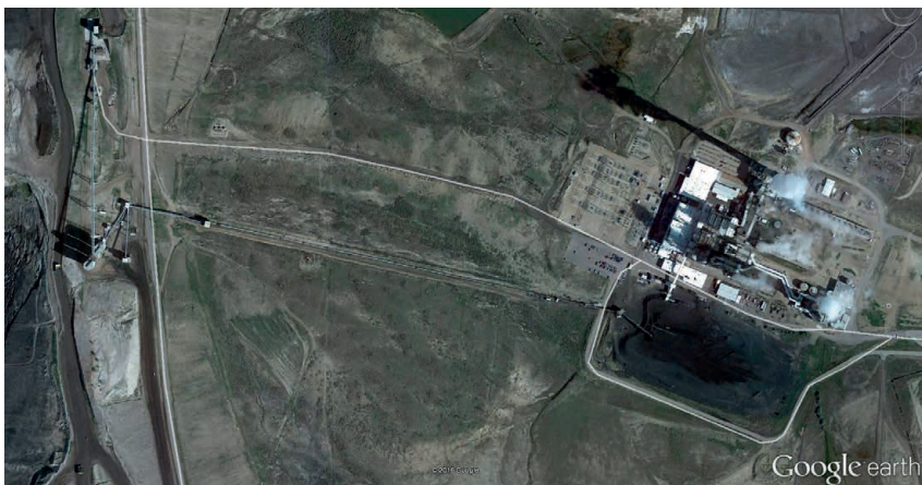
Figure 2. Westmoreland Kemmerer mine (left) and thermal power plant (right) are connected by 4200 ft long overland conveyor, which moves 2.8 million tpy of sub-bituminous coal.
