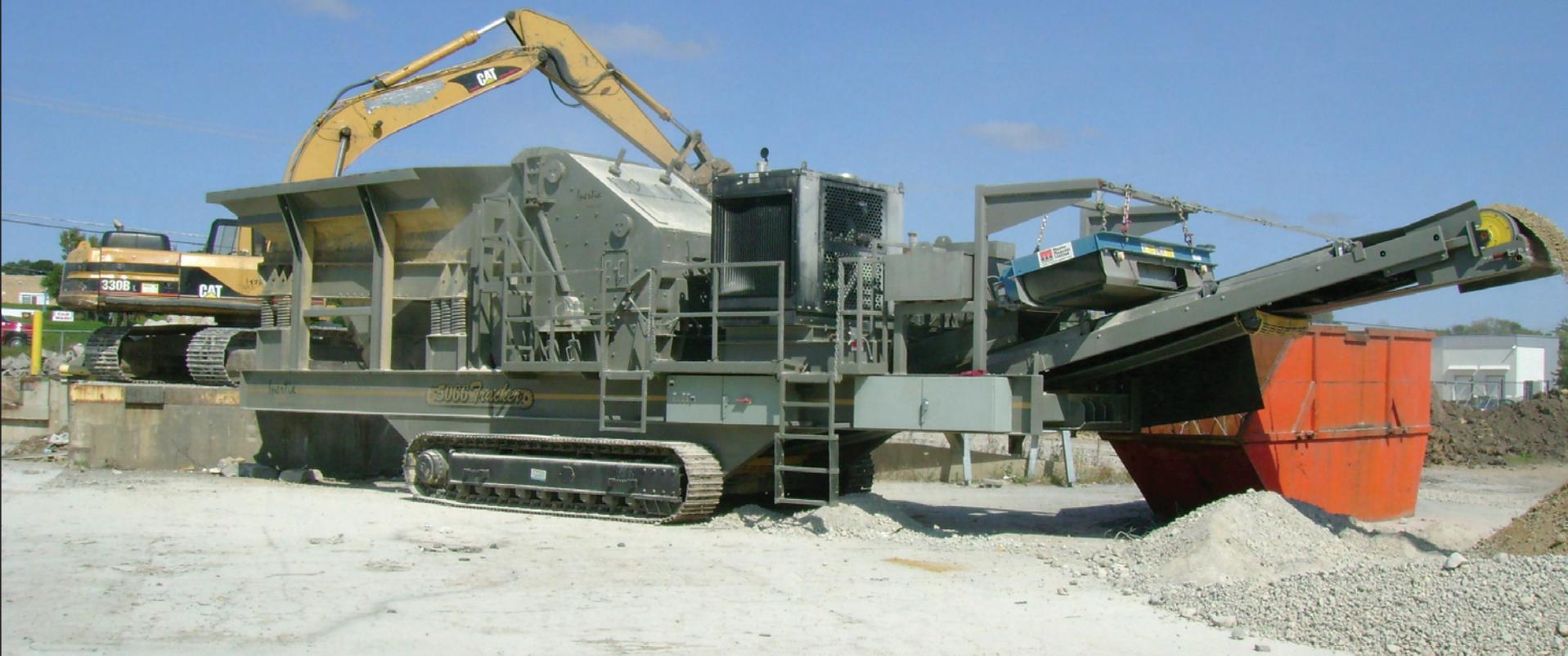
**5066 Tracker diesel engine drives crusher, hydraulic pumps for tracks and clutch and generator for all electric motors.**
