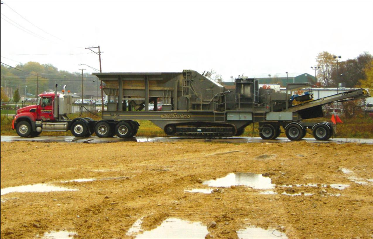
**5066 Tracker features quick and easy transport capability using built in three axle bogey.**
