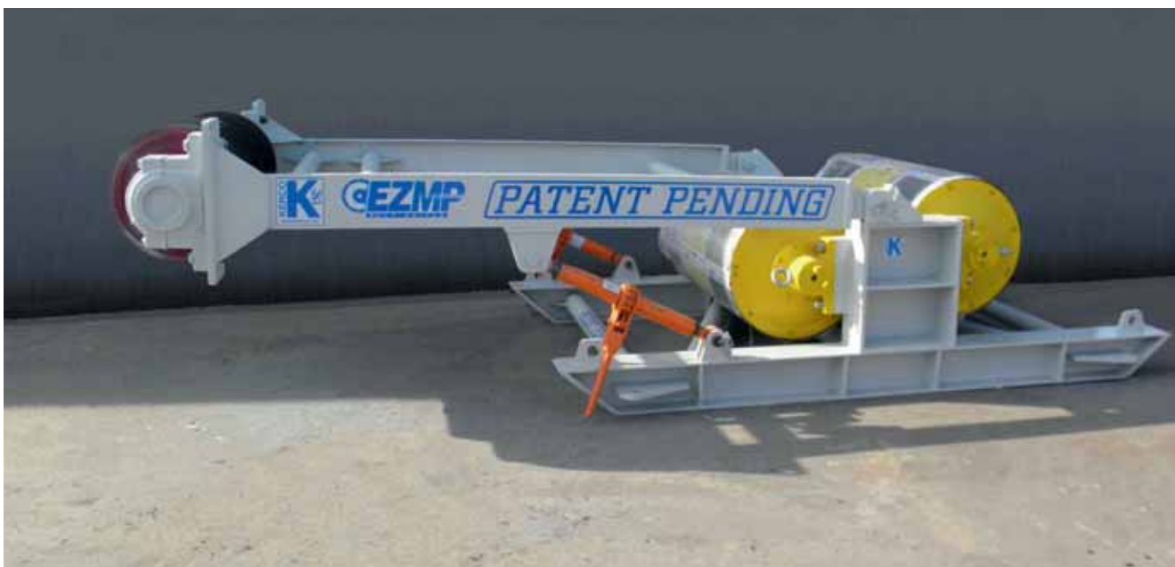
Built for underground coal mines, Kercó's 150 HP EZMP drive includes two model 630H 75 HP Rulmeca motorized pulleys and may be mounted to mine floor or ceiling. Optional boom converts system from booster to discharge end drive. EZMP drive systems up to 660HP are available.
