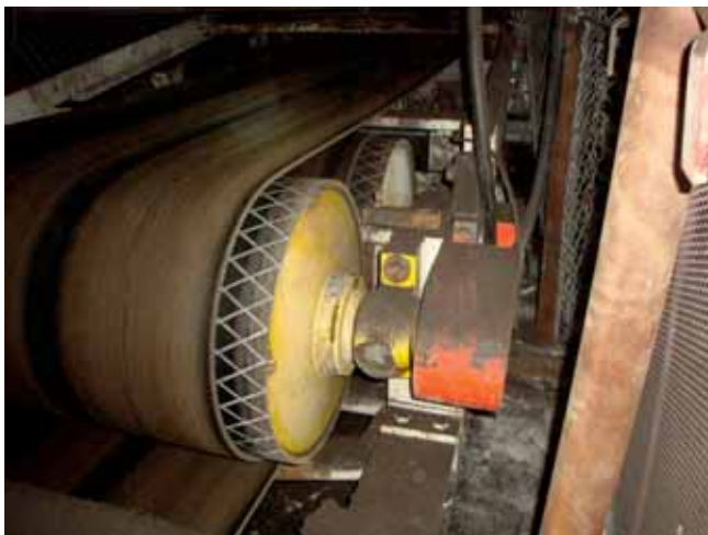
Model 630H motorized pulley has narrow footprint (24.8" diameter and 55.12" face width.) Each drive only weighs 2,200 lbs. Drive compactness and light weight are advantageous when moving conveyor in restricted spaces underground.
