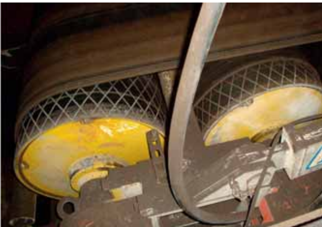
Two model 630H 75 HP Rulmeca Motorized Pulleys in 'nested dual' arrangement. Note the absence of external motor, gearbox, and pillow blocks. All mechanical components are hermetically sealed within the pulley's oil-filled shell.
