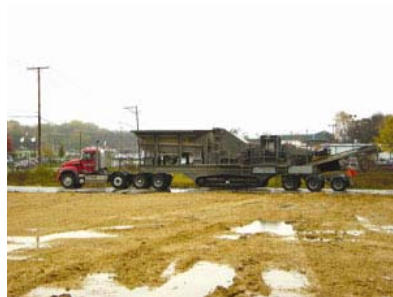
5066 Tracker features quick and easy transport capability using built in three axle bogey.
