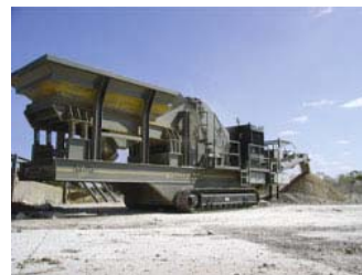
Inertia Machine's 5066 Tracker features Rulmecca Motorized Pulley model 400M at 15 hp to move up to 700 tph of crushed product at 300 fpm, using 460v/3ph/60Hz.
