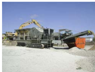
5066 Tracker diesel engine drives crusher, hydraulic pumps for tracks and clutch and generator for all electric motors.
