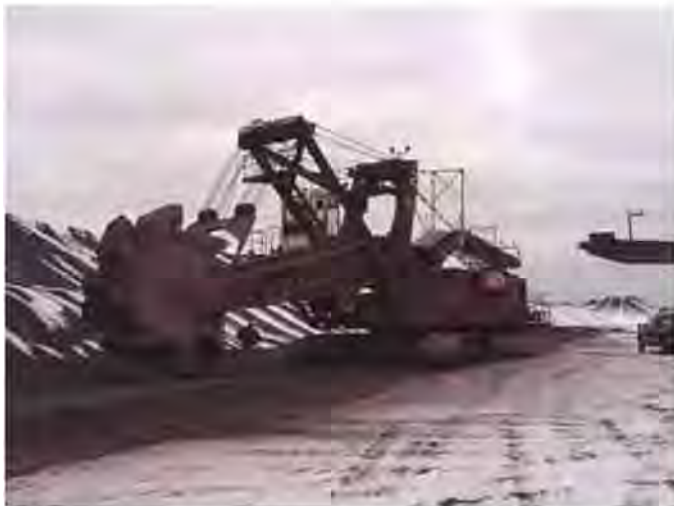
Photo shows one of three 40 year old bucket wheel reclaimers outfitted with 100 HP Rulmecca Motorized Pulleys. In addition to improving reliability, dual drive system on tail conveyor extended belt life since its 2004 installation.
