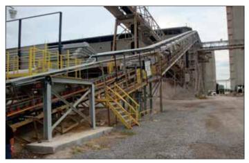
This US cement producer eliminated 4' of start-up belt bounce and subsequent belt and feeder damage on their concave reclaim tunnel conveyor when they upgraded from a 75 HP head pulley to two 50 HP Motorized Pulleys in the head and tail positions. The 360° of belt wrap decreased slack side tension and enabled the operator to use the existing belt in spite of the fact that installed power was increased by 33%.
