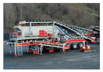
Driving cross belts, screen feeds, recirc belts, hopper feeders, transfer conveyors, and belts under screens and crushers, Rulmeca Motorized Pulleys are used on crushing/screening plants, stackable conveyors, radial stackers, reversing shuttle conveyors, and miniature conveyors in aggregate and frac sand production, highway construction, mining, and recycling.
