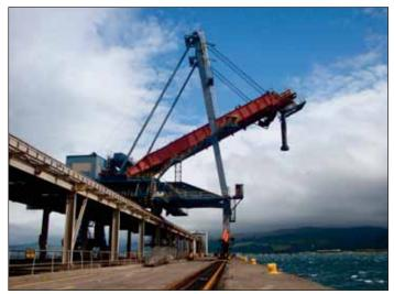
Located in Scotland, this major coal transfer terminal has installed model 800HD and 1000HD Rulmeca Motorized Pulleys on the dock (330 HP), in the ship loader (2 x 180 HP) and in the rail loadout system (2 x 100 HP), taking advantage of the thermal characteristics of the drives. Since Rulmeca Motorized Pulleys dissipate motor heat into the belt, some operators consider Motorized Pulleys to be "belt warmers," which is an advantage in winter weather.
