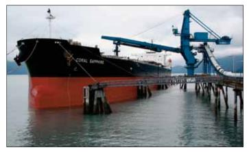
This Alaskan rail-to-ship transfer terminal installed a 75 HP 24.8" diameter Motorized Pulley in the ship loader shuttling boom conveyor when they upgraded the machine to handle 2,000 tph of coal. Faced with frigid conditions, the operator chose the optional anti-condensation heater, which maintains a constant warm temperature within the pulley shell when the machine is idle. Other operators use "trickle voltage" heating to serve the same purpose.
