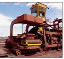
Pulleys at the head and tail positions, with electronic load-sharing, eliminated the problem on this reversing shuttle belt, which feeds the 60 ship loader surge bins. A close up of the west end drive is shown.
