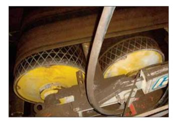
With a light weight of 8,600 lbs. and an overall width of 78", these two 75 HP, 24.8" diameter Motorized Pulleys move coal underground at 1,200 tph on a 48" wide conveyor more than 1,200'. Easy to relocate and safer than an exposed drive system, this is an ideal dual drive.
