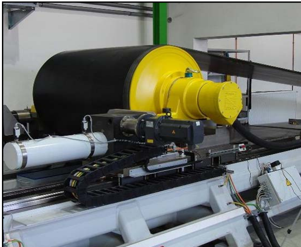
Figure 15 Photos show model 1000HD (left) at 330 HP under full load testing at Rulmeca Germany GmbH facility in Aschersleben, Germany. Test chamber (right) includes capability to monitor all important electrical, thermal, and noise design parameters.
