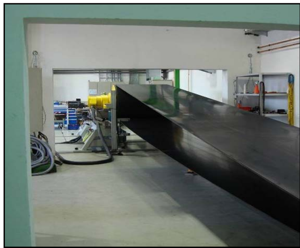
Figure 15 Photos show model 1000HD (left) at 330 HP under full load testing at Rulmeca Germany GmbH facility in Aschersleben, Germany. Test chamber (right) includes capability to monitor all important electrical, thermal, and noise design parameters.
