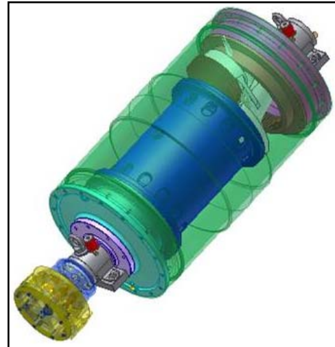
Figure 16 CAD drawing illustrates features which are essential to enable flameproof capability and certification
