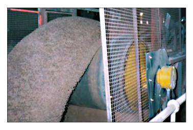
In 1999, this quarry replaced a single 100 HP drive on its reversing shuttling conveyor with two 50 HP Motorized Pulleys, one in the head position and one in the tail position. This 24.8" diameter model 600H dual drive system eliminated belt tracking problems and significantly extended belt life, thanks to 360° of belt wrap and lower slack side tension. It is also possible to add power to an existing conveyor by replacing an appropriate idler pulley with a Motorized Pulley.
