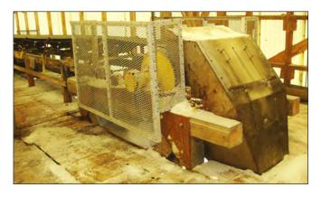
Enclosing the drivetrain within a hermetically-sealed, oil-filled pulley shell makes the drive compact and protects
