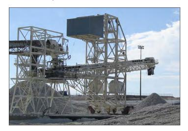
Belt wrap was increased from 180° to 360° at this western US trona mine by the adding a 60 HP, model 630H, 24.8" diameter Motorized Pulley to the head of this 40-year-old radial stacker. It eliminated slippage of the 100 HP tail drive during rainy conditions. The 2,400 lb. Motorized Pulley replaced a 3,200 lb. idler pulley, requiring no structural modifications to the stacker truss.
