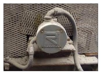
One of numerous Rulmeca Motorized Pulleys used by major US salt producers, this unit dramatically reduced maintenance expense while increasing conveyor drive reliability. The mine eliminated the need to grease external bearings and replace corroded drive components while reducing the oil change frequency to 50,000 operating hours by using synthetic oil. That equates to an oil change every six years, based on a "24/7" operating schedule.
