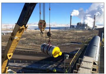
This Wyoming coal mine upgraded their overland conveyor feed system with a 150 HP, model 800H, 31.5" diameter Motorized Pulley. Faced with frigid conditions, some operators choose the optional built-in anti-condensation heater, which maintains a constant warm temperature within the pulley shell when the machine is idle. Other operators use "trickle voltage" heating to serve the same purpose.
