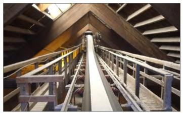
This Midwest US salt mine reduced belt bounce and eliminated a flat catenary and subsequent material spillage at the tripper in their raw salt storage shed loading conveyor by replacing one worn 40 HP head drive with two new stainless steel 20 HP, model 400M, 15.75" diameter Motorized Pulleys in the head and tail positions.
