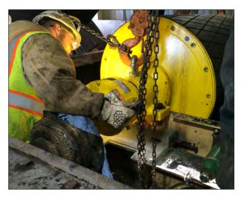
With a light weight of 5,100 lbs. and overall width of 91", this 150 HP, model 800H, 31.5" diameter Motorized Pulley moves coal from a western US coal mine directly to a power plant overland conveyor. This is an ideal primary conveyor drive because reliability is essential.
