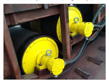
Great Lakes rail-to-ship transfer terminal extended discharge belt life by decreasing slack side tension. A serpentine belt wrap angle of 420° produced by the two 31.5" diameter model 800H Motorized Pulleys made this possible. More than fifteen years of successful operation have confirmed that belt life has been extended.
