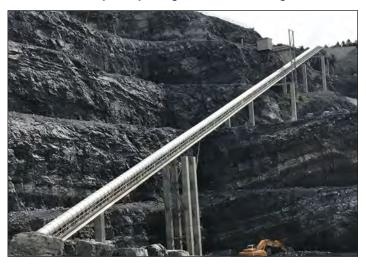
This US limestone producer reduced maximum belt tension at the discharge (head) pulley from 27,000 lbs. to 17,000 lbs. after modifying his conveyor drive design from a single 300 HP drive with a 384 fpm belt speed to a dual drive with a 600 fpm belt speed. This will yield a significantly longer belt life because of reduced belt stress. Each of the two drives was a 150 HP, model 800H, 31.5" diameter Motorized Pulley controlled by load-sharing VFDs.
