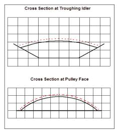
Plot shows that selected belt speed (dotted line) may cause material spillage because cross section exceeds CEMA recommendation (solid line.)
