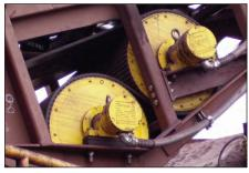
Hermetically sealed carbon steel tube and end housings with standard paint are suitable for most bulk applications. However, aggressive environments may require regreasable seals, special finish, or stainless steel. See pages 86 - 87.
