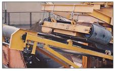
Certain applications (e.g. self-cleaning electromagnet for tramp iron, pictured above, "tilted" package sortation conveyors, and "travelling wall") require pulley shaft to be mounted out of the horizontal plane. This Motorized Pulley option requires extra oil, grease packed top bearing, and special electrical termination. Contact Rulmeca for assistance. see pages 84, 86, and 91.
