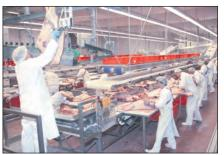
Environments with high amounts oil, grease, and/or fat require special oil-resistant lagging. If they require frequent high pressure and/or chemical cleaning they may also require regreasable seals and stainless steel or special surface coating. See pages 82 and 87.
