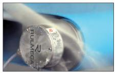
Regreasable seals, full stainless steel, and food grade oil, grease, and lagging material are suitable for this environment, which usually includes frequent high pressure/chemical wash down. See pages 82, 83, & 87.
