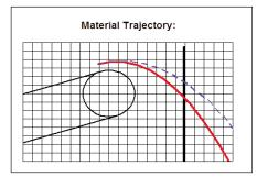
Trajectory plot shows that slower belt speed (solid line) will not plug chute while faster belt speed (dotted line) will. This is because trajectory of center of material mass impacts against vertical chute wall above horizontal centerline of pulley.
