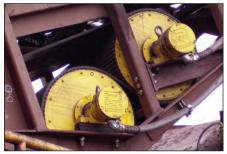
Hermetically sealed carbon steel tube and end housings with standard paint are suitable for most bulk applications. However, aggressive environments may require regreasable seals, special finish, or stainless steel. See pages 88-89.
