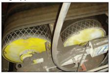
Rulmeca Motorized Pulleys have been incorporated into underground mining and tunnel boring machines. However, they are not "intrinsically safe" or "flame proof" and are not suitable for service where explosive gasses, vapors, liquids, or dust are continuously present. Contact Rulmeca for additional details.
