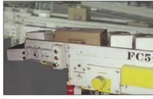
Electromagnetic brake provides excellent product "hold" capability in induction systems requiring "indexing." See pg 83-84.
