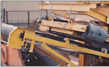
Certain applications (e.g. self-cleaning electromagnet for tramp iron, pictured above, "tilted" package sortation conveyors, and "travelling wall") require pulley shaft to be mounted out of the horizontal plane. This Motorized Pulley option requires extra oil, grease packed top bearing, and special electrical termination. Contact Rulmeca for assistance. see pages 86, 87, 88, and 93.
