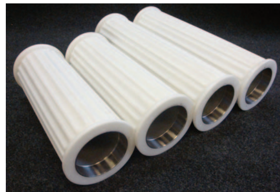
Top: Stainless steel shells profiled to drive smooth continuous positive drive belt
