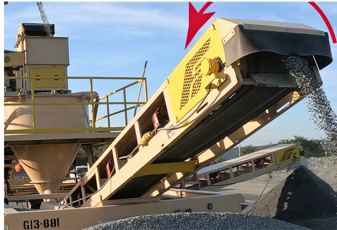
Figure 5. Motorized pulley transfers conveyor belt drive torque directly into structure, eliminating structural twisting during start-up.
