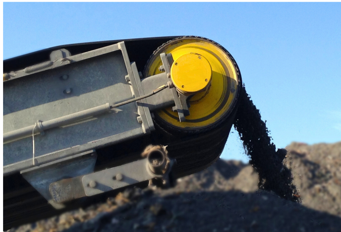
Figure 3. Motorized pulley (15 HP) driving 36-inch wide bottom ash discharge conveyor on portable metal recycling system at US waste-to-energy power plant.
